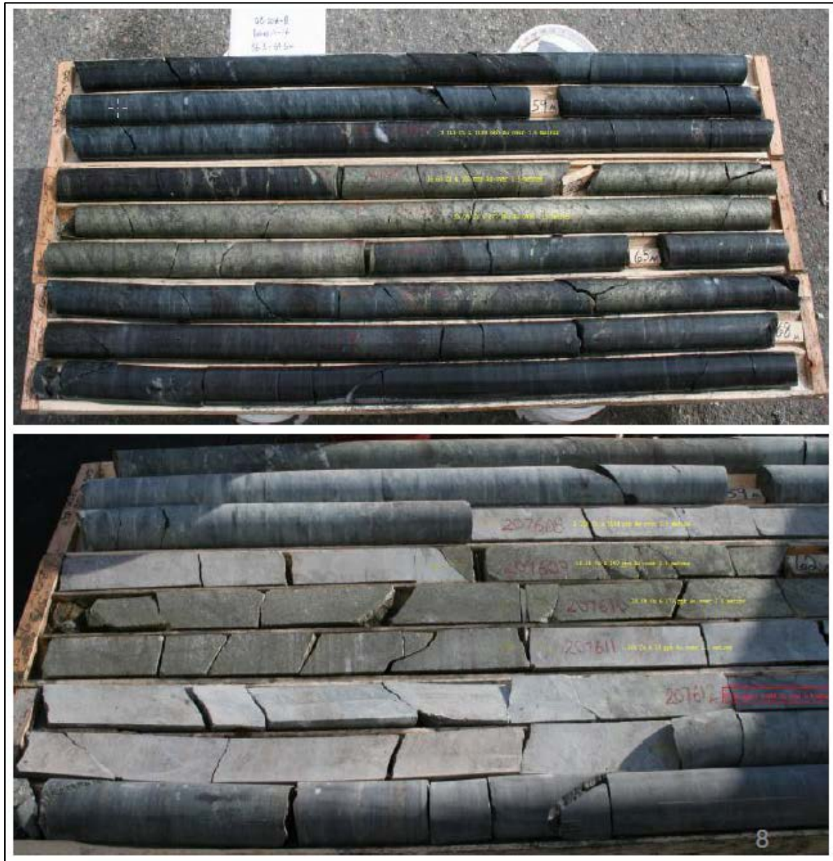
FIGURE 7.5 MASSIVE SULPHIDE INTERSECTION FROM 2016 DRILL HOLE GB-01-07 IN GREAT BURNT COPPER DEPOSIT
