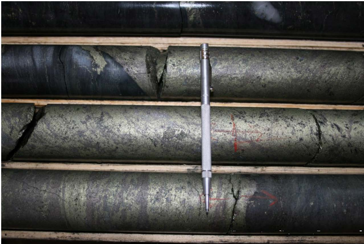
FIGURE 10.3 CLOSE-UP PHOTOGRAPH OF MASSIVE SULPHIDE MINERALIZATION IN DRILL HOLE GB-16-8
